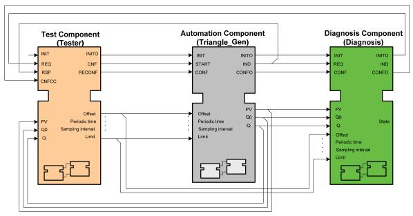
Figure 6: Sample Application with applied Function Blocks in IEC 61499.
