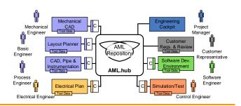
Exchanged engineering data will become easily accessible in tool networks using the open *AutomationML* (AML) data exchange format with the *AML.hub*. The *AML.hub* enables step-wise migration to *AML*-based engineering projects.
