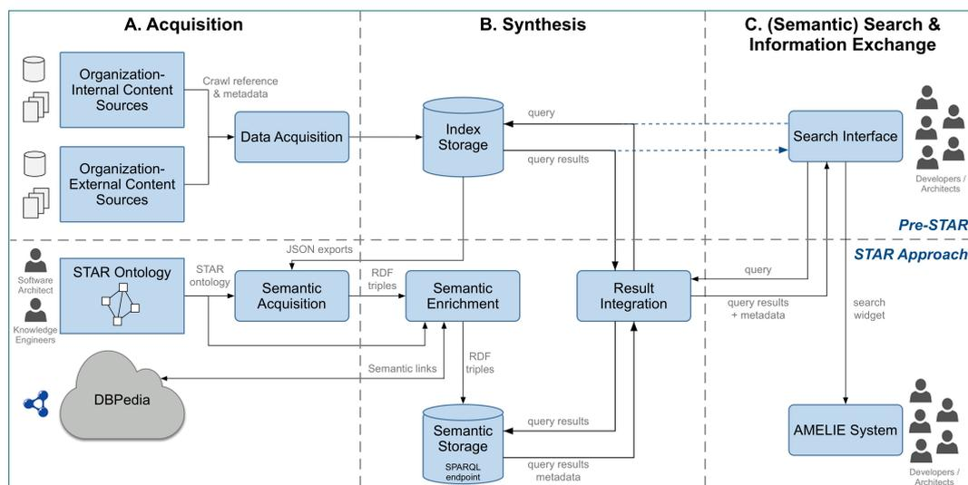
Figure 1 Extension of a keyword-search system into a semantic exploratory system with the STAR approach.
