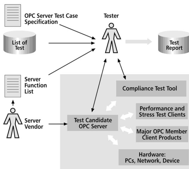
Figure 1: Overview on OPC-UA Protocol Testing<sup>2</sup>
